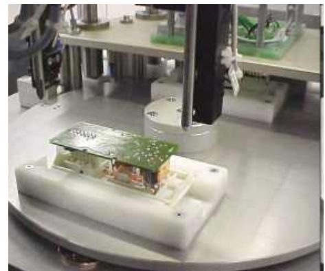
180° Indexing Table with Specimen Mount
